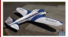
Launched in 1933, the Boeing 247 was the first to pioneer what would later become the basic formula in the industry: all-metal construction, low cantilever wing and retractable landing gear. Despite this, its capacity and performance couldn't compete with the Electra or the DC-3, and only 75 were built. Four survive as of 2020, one airworthy.
